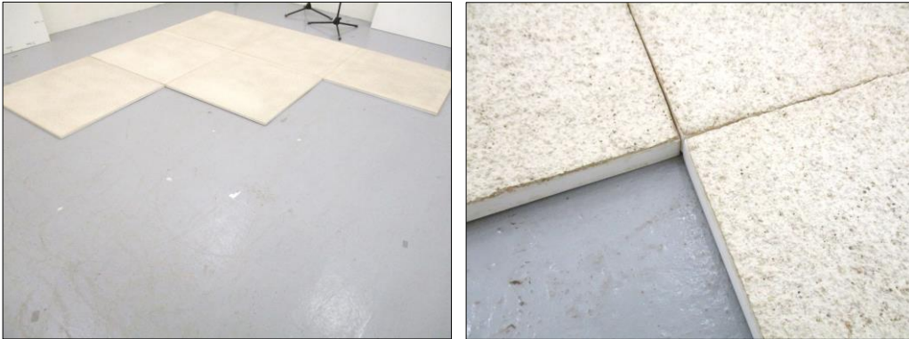
Images 3 and 4 Assembly of the test sample in the reverberating room
